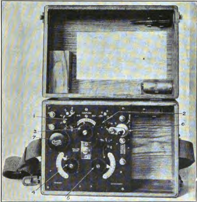
FIG. 252.—Simple receiving set (Signal Corps Type SCR-54-A), portable cabinet type.
